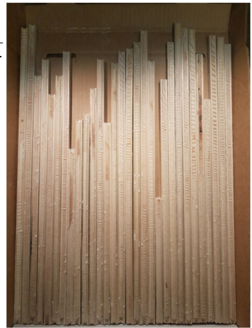
Mounted and sanded tree cores awaiting ring width measurement in the Nevada Paleoenvironmental Analysis Laboratory at UNR.
