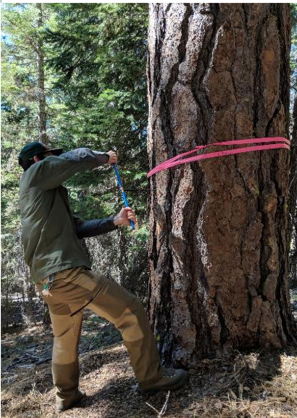
Ben turns an increment borer to collect a tree core from a focal tree in the unthinned forest.
