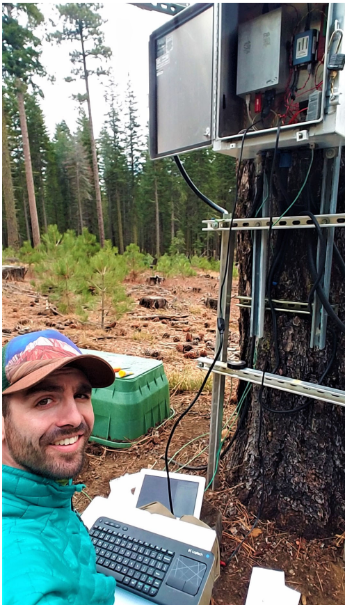
Ben performs a routine maintenance check up on the wireless data collection network and central field computer, located in the Group Select.
